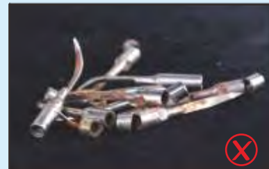
After working 6 minutes, Tips of poor quality started to crack, after 12 hours, all the tips are cracked
