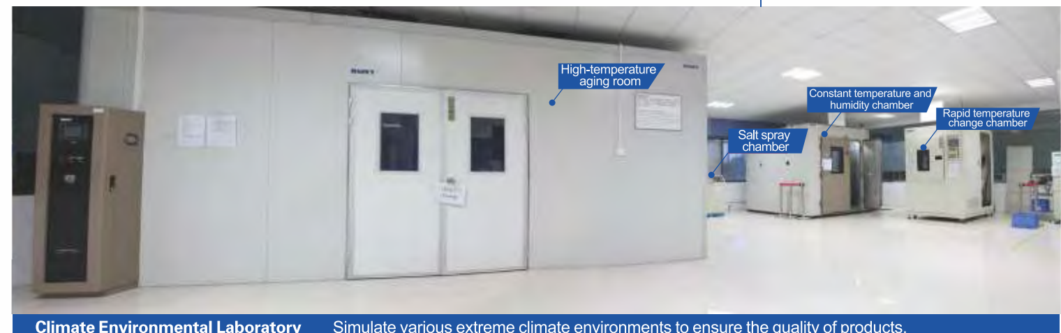
Climate Environmental Laboratory Simulate various extreme climate environments to ensure the quality of products.
