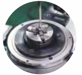
Roundness measuring instrument imported from Japan, high degree of accuracy(0.01um)
