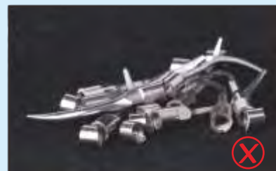
Tips of poor quality start to be cracked after one-hour working, the cracking rate within 10 hours is 35%.
