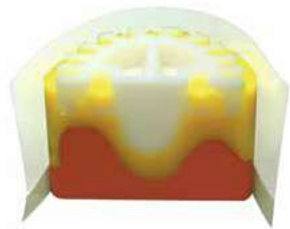
Cross-section of a flaskless duplicating mould
